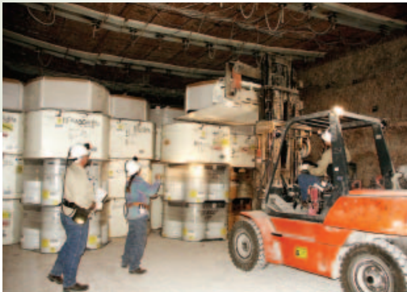
Transuranic waste is stacked in a disposal room 2,150 feet underground.
